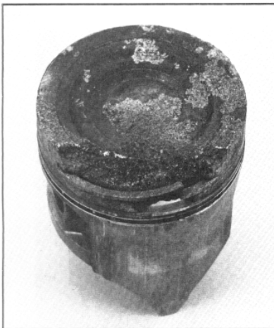
Melted top land, sheared secondary lands.
