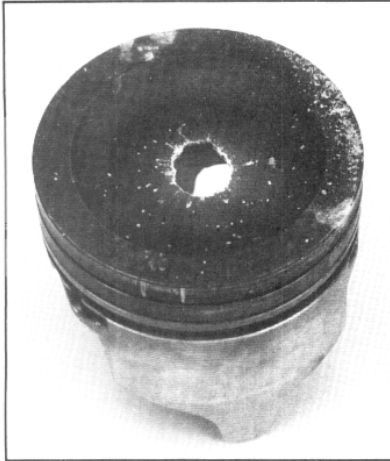
Damage to piston head.
