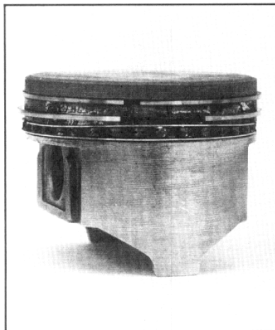
Secondary land damage indicates extreme temperatures and pressures.
